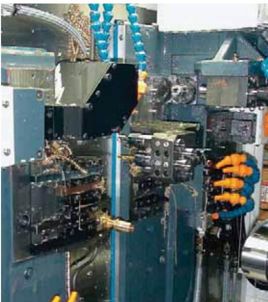
Swiss ST 26 making a connector body.
