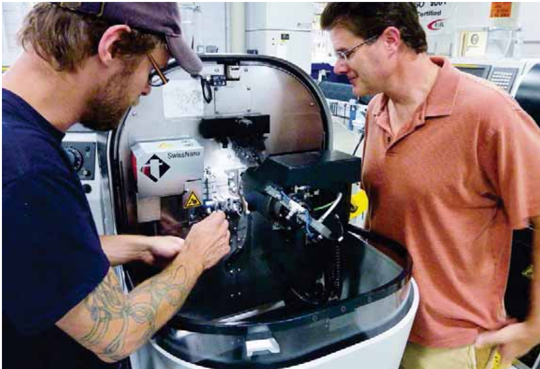
Petron's CNC Manager and Plant Manager fixing a 7-degree angle block in one of the new SwissNanos to manufacture a custom part for the Medical and Electronics industries.
