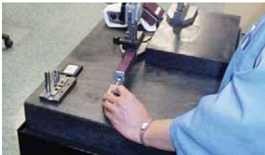
Quality Control engineers using a Profilometer to check ID finish for a part made in one of the EvoDeco 32.
