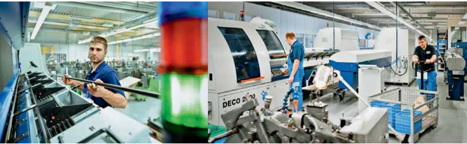
Always state-of-the-art technology: Laufer's machinery consists almost exclusively of the latest Tornos CNC single spindle and CNC multi-spindle automatic lathes.
